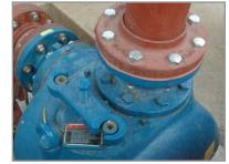
Equal in importance to maintenance is safety. The WSP<sup>TM</sup> self-primer pump is designed with the added benefit of the Fill Port Cover and Clamp Bar Assembly. The recessed bolt-locking construction and anti-rotation design of the Clamp Bar Assembly prevents accidental breach of the Fill Port Cover, protecting the operator from scalding burns.
