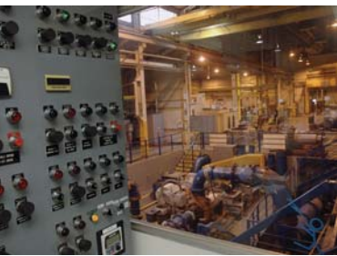
Photos: Above, Engineering test facility control room. Bottom right, Roto-Jet pumps being tested in high-pressure engineering test facility.
