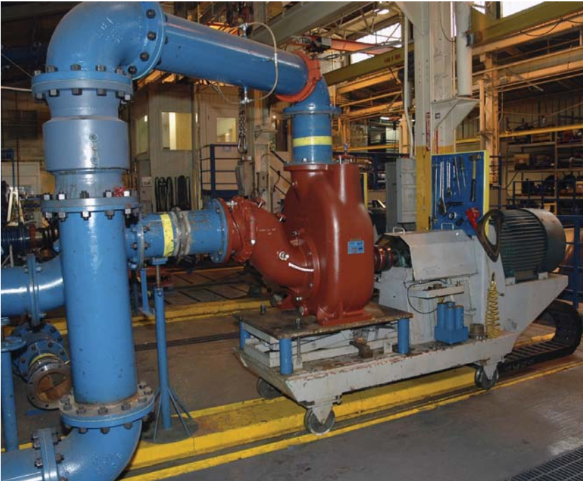
Photos: Above, WEMCO Self-Primer on test cart. Top right, Large horizontal & vertical pump test area. Middle right, Pumps being tested. Bottom right, Customer witness area in control room. Bottom left, large centrifugal pump package being tested.
